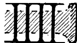
Fig. 20 —Diagram of the Milling and End Section of a Shilling of Edward VII, 1906, to shew raised milled edge which largely prevents the rubbing or wearing away of the two faces.
